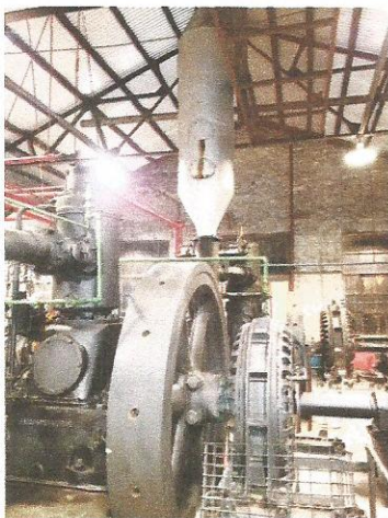
This little fellow is called Unit #2. It is only a 50hp single cylinder diesel engine. It was an experience watching Tony fire it up.
