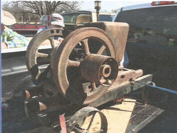
Rated at about 3hp, this unit is referred to as a “headless” Fairbanks-Morse engine.
