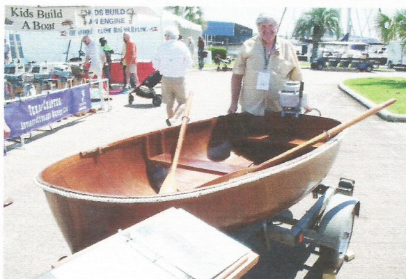
Paul Johnson standing by his 1941 Skaneateles Hydro-Lite cedar strip dingy and its 1939 Johnson LT-39 Light Twin 5hp outboard.
